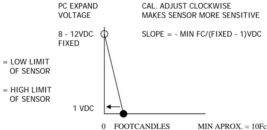
The max fixed VDC is the maximum voltage the sensor can output. This can be as High as 12VDC, but is normally 10VDC, which is what we will use here and always. Hence the equation for our example becomes:
