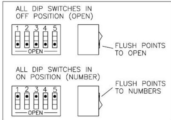
Figure 5A: Timer Switch Diagram
