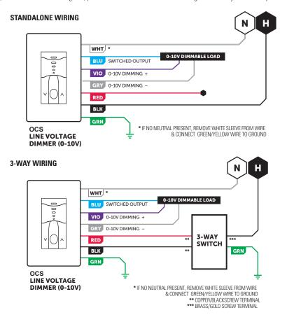
NOTE: This product is UL listed and meets NEC 404.2(c) & 404.22 guidelines regarding powering over ground & current leakage. Powering over ground is permitted for replacement / retrofit only.
