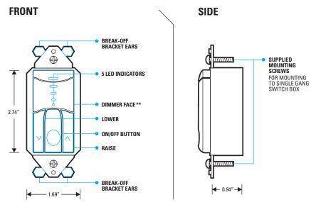
\*\* SENSOR FACE IS FIELD REMOVABLE IN ORDER TO CHANGE COLORS. CONTACT FACTORY FOR ADDITIONAL FACES
